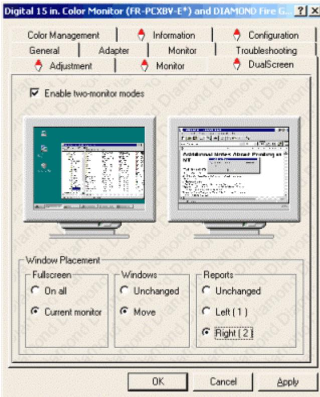
2. Select **Enable two-monitor modes** to enable screen resolutions for a two-monitor configuration in the **Settings** dialog. Deselecting this option will allow single-monitor resolutions only.
