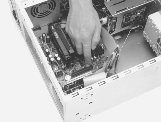
2. Remove the metal slot covers from the AGP slot and the adjacent slot. Save the screws to secure the graphics card later.
