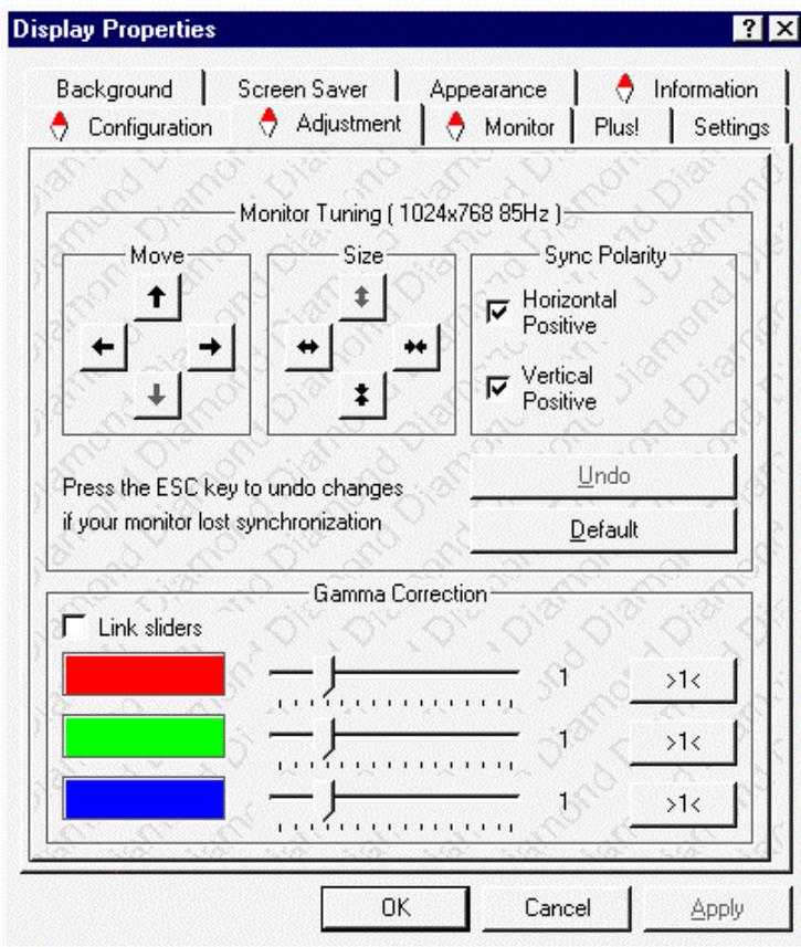
2. **Monitor Tuning:** With the buttons in the **Move** and **Size** sections you can tune the position and size of the monitor's display for the indicated resolution and refresh rate.
