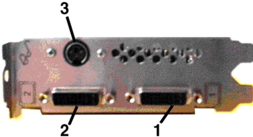
**i** **Note:** If the connector on your stereoviewing eyewear does not fit into the Mini-DIN connector on the card, please contact your supplier or the manufacturer of the stereo glasses for information on how to obtain an adapter cable.
