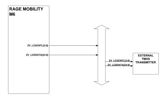
Figure 39: External TMDS support
