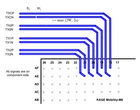
Figure 32: Routing TMDS Lines
