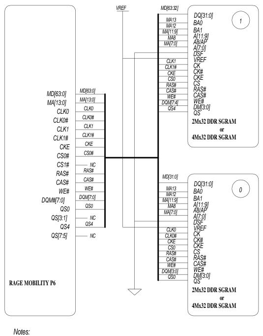
For 8MB 32 BIT Interface install 0 of type 2Mx32 For 16MB 64 BIT Interface install 0, 1 of type 2Mx32 For 16MB 32 BIT Interface install 0 of type 4Mx32 For 32MB 64 BIT Interface install 0, 1 of type 4Mx32 \*MA11 is needed only for the 4Mx32 part
