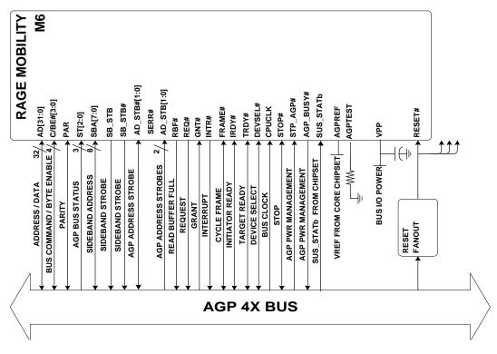
Figure 5: AGP Interface Block Diagram
