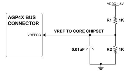
Figure 6: VREF Voltage Divider Circuit
