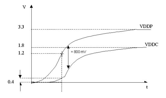
Figure 4 Power sequence when VDDC derives from VDDR
