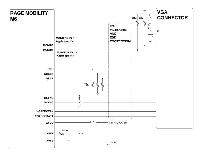
Figure 31: Analog Display Section
