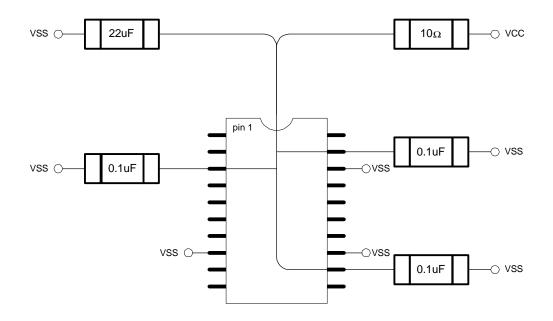
Figure 41: SM530 Single Power Plane Layout
