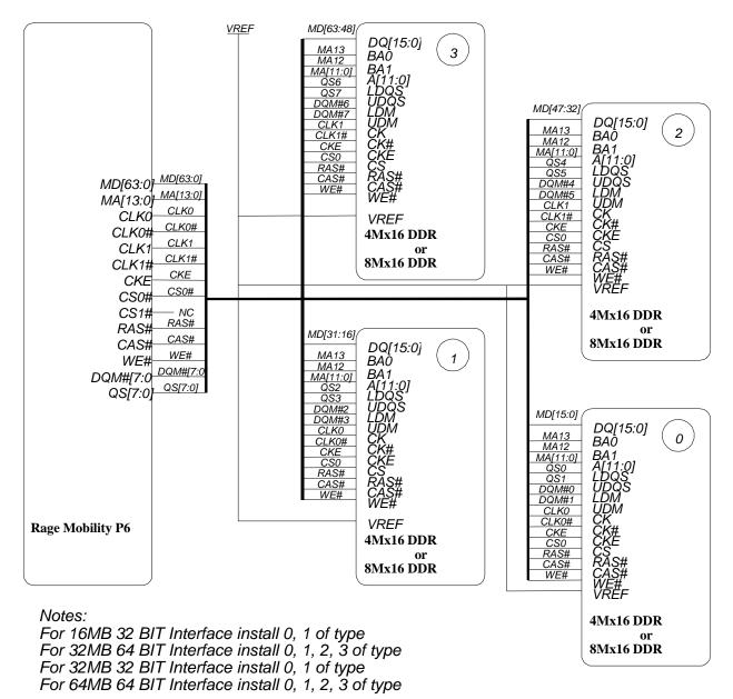
Figure 14 DDR SDRAM Configuration
