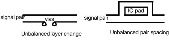
Figure 33: Avoid Unbalanced Layer Change
