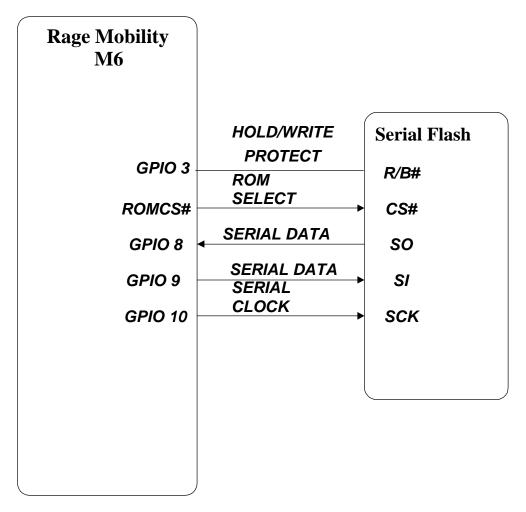
Figure 27: BIOS Interface – Serial EEPROM Configuration
