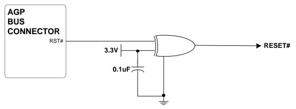
Figure 7: RESET Buffer Circuit
