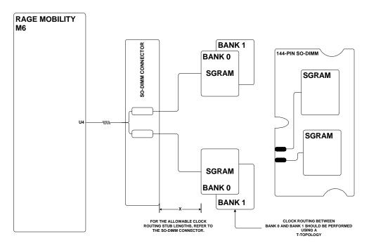
Figure 19: Memory Clock Routing
