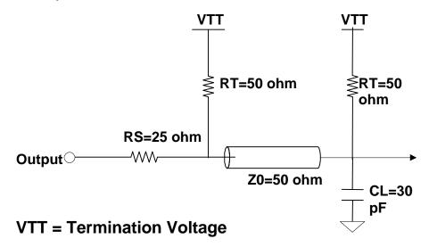
Figure 24: Class II SSTL-2 DDR termination
