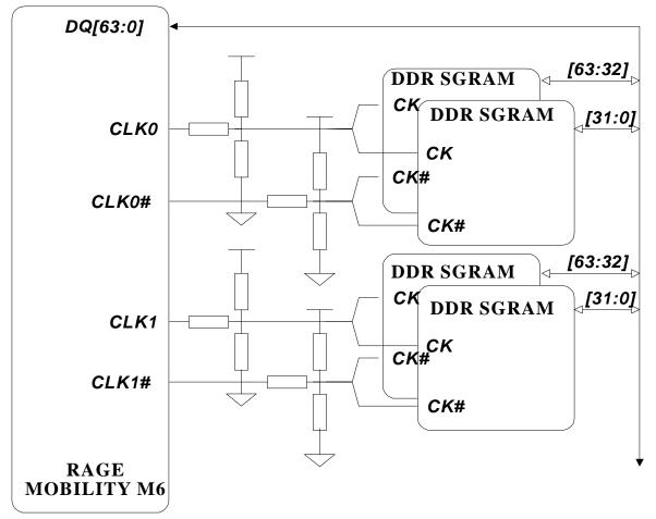
Figure 17: Memory Clock: Termination and Distribution for the 64-Bit DDR
