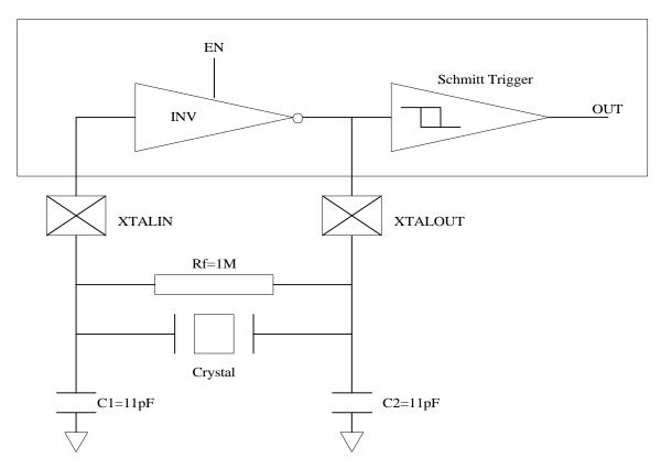
Figure 30: Oscillator Circuit
