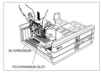
Grasp the card by the top edge and carefully seat it firmly into the PCI slot.
