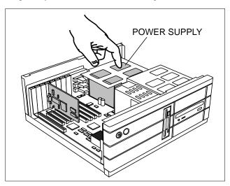
Remember to discharge your body's static electricity by touching the metal surface of the computer chassis.
