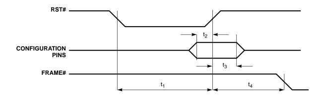
Figure 6-9. RESET Timing
