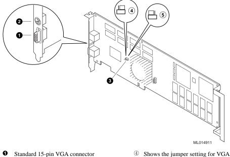
Figure 3-1 PowerStorm 350 PCI Graphics Controller
