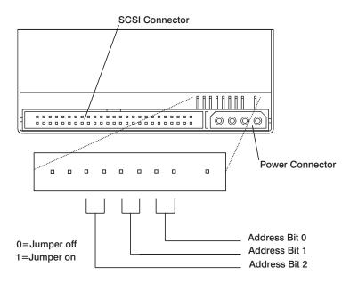
There are two pins for each bit. When a jumper is on (shorting two pins together) that represents a 1 in the following SCSI ID table. The three bits in the ID give a range of 0 through 7 as follows:
