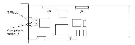
The Ultimedia Video Capture Adapter allows connection of the system unit to various video equipment.
