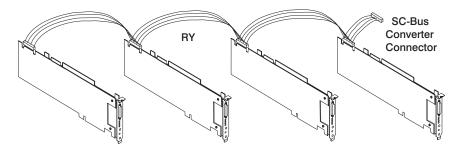
H.100, 4-Drop cable with SC-Bus Converter Connector
