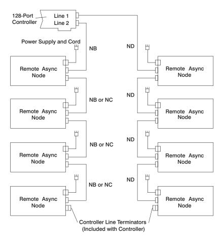
A choice of cables can be attached to any of the 16 Remote Async Node ports. See the following illustration. These ports are labeled 0 through 15 and accept 4-, 6-, 8-, and 10-pin RJ-type connectors.
