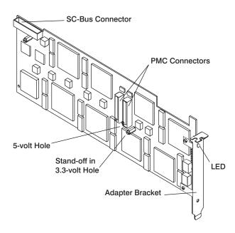
The IBM ARTIC960Hx DSP Resource PCI Adapter connects to the ARTIC960Hx Base Adapter by two 64-pin connectors. See "PMC Connector" on page 175. The interface signals exit the DSP Resource PCI Adapter through the 26-pin signal-computing bus (SC-bus) connector at the top of the PCI Adapter. The IBM ARTIC960Hx base adapter and the attached DSP Resource Adapter occupy a single full-size 32-bit PCI expansion slot.
