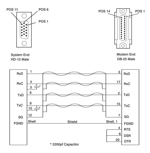
The 128-port async controller supports multiple controller line baud rates in EIA-232 synchronous-modemattach mode. Although the 128-port async controller can operate at 57.6 Kbps, to ensure a low error rate on the synchronous link, controller line baud rates of 19.2 Kbps or less are recommended.
