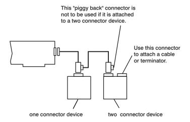
A dedicated adapter is recommended for attachment of any external enclosure containing multiple SCSI devices.
