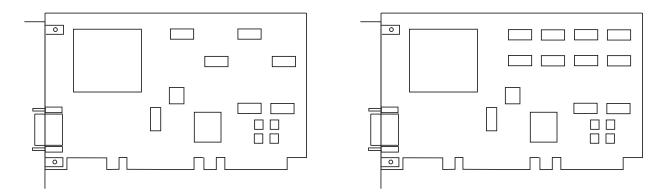
**Note:** In the illustration above, the GXT250P is on the left side and the GXT255P is on the right. The GXT255P has more modules in the upper-right quadrant of the adapter.
