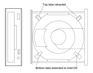
Note: All four tabs must be retracted when the drive is used horizontally.
