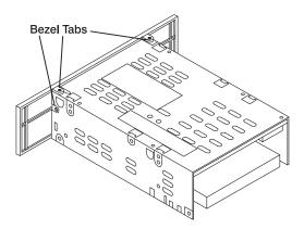
b. Place the drive assembly on its right side. Facing the drive assembly, use a small screwdriver to gently press on the bezel tab (through the rectangular hole in the drive assembly). Continue to press on the bezel tab until the latch on the bezel tab clears the hole and the bezel can be pulled away from the drive assembly.
