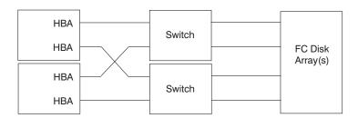
The following illustration shows an example of a high-availability cascaded switch configuration. In this example, four switches are cascaded in such a way that if any one switch port (or even one whole switch) fails, the remaining three switches still form a fully functional fabric.
