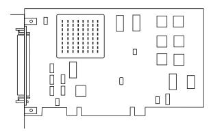
The attachment adapter feature allows connection of the system unit to a 7250 POWER GXT1000 Graphics Accelerator.
