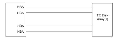
**Hub Configurations:** One or more hubs can be included in a Fibre Channel configuration allowing a host system HBA and one or more Fibre Channel devices to be connected in a Fibre Channel Arbitrated Loop (FC-AL) topology. Hubs can be cascaded, that is, a port of one hub can be connected to a port of another hub.
