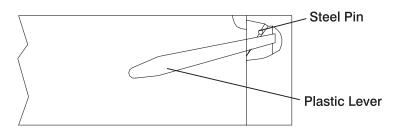
Attention: When attaching the bezel, the cassette door must be raised to make sure that the steel pin on the left side of the door (with the drive assembly facing you) is above the white plastic lever on the left side of the drive assembly.
