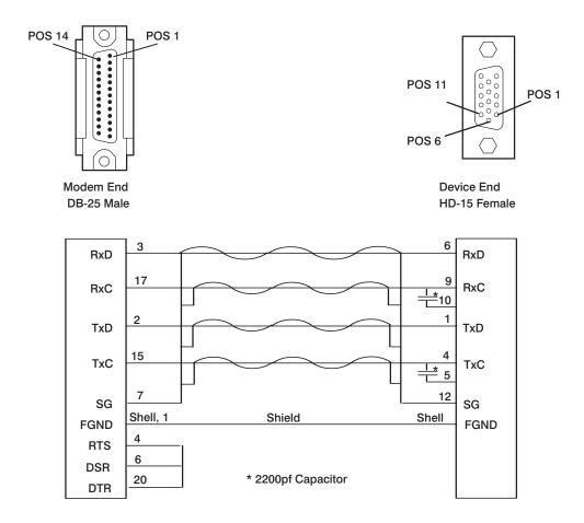
The 128-port async controller supports multiple controller line baud rates in EIA-232 synchronous-modemattach mode. Although the 128-port async controller can operate at 57.6 Kbps, to ensure a low error rate on the synchronous link, controller line baud rates of 19.2 Kbps or less are recommended.
