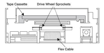
After the tape drive guidance rollers have fully retracted, turn the drive so that you are facing the front. With a small non-magnetic probe, access one of the drive reel sprockets and manually rotate the drive reels until all of the tape has been wound inside of the cartridge.
