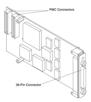
The IBM ARTIC960Hx 4-Port Selectable PMC connects to the IBM ARTIC960Hx base adapter by two 64-pin connectors. See "PMC Connector" on page 175.Interface signals exit the 4-Port Selectable PCI Mezzanine Card through the 120-pin connector at the rear of the card. The IBM ARTIC960Hx base adapter and the attached 4-Port Selectable PMC occupy a single 32-bit expansion slot.
