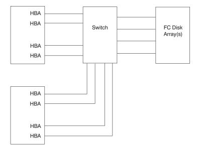
Switch Configuration with Four Host Systems: The following illustration shows an example of four host systems connected through a switch to a Fibre Channel disk array.
