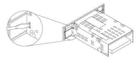
c. Move the bezel aside to provide access to the front of the drive assembly.
