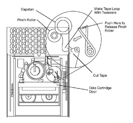
3. Make a loop in the tape with the tweezers, and cut the tape as indicated in the preceding figure.
