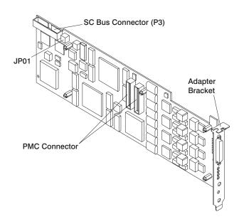
This IBM ARTIC960Hx 4-Port T1/E1 Mezzanine Card connects to the IBM ARTIC960Hx Base PCI Adapter by two 64-pin connectors. See "PMC Connector" on page 175. The interface signals exit the 4-Port T1/E1 Mezzanine Card through the 36-pin connector at the rear of the card. The IBM ARTIC960Hx Base PCI Adapter and the attached 4-Port T1/E1 Mezzanine Card occupy a single full-size 32-bit PCI expansion
