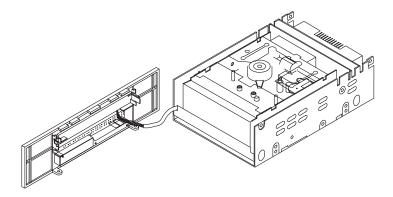
4. Turn the mode motor shaft counterclockwise until the mode motor stops.
