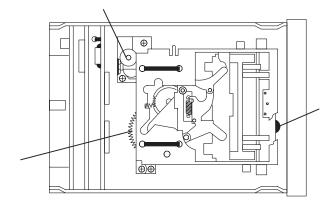
5. Push the front roller in and turn it clockwise until the tape is wound on the supply reel, and the roller stops.
