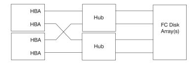
Hub Configuration With Four Host Systems: The following illustration shows an example of four host systems connected through a single hub to a Fibre Channel disk array. This example also illustrates the maximum of seven connections available on a hub.
