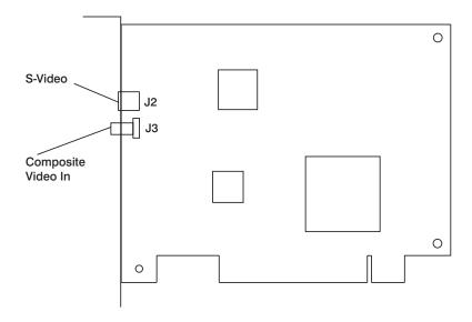
The Ultimedia Video Capture Adapter allows connection of the system unit to various video equipment.
