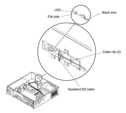
FIGURE 8-24 Removing/Replacing the Speaker/LED Cable
