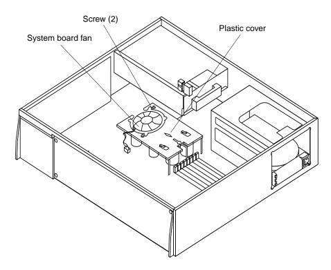
FIGURE 10-24 System Board Fan Plastic Cover
