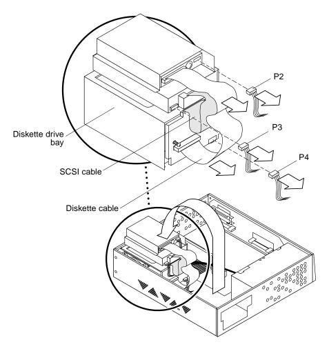
FIGURE 8-18 Removing the Peripheral Power Cable Connection
