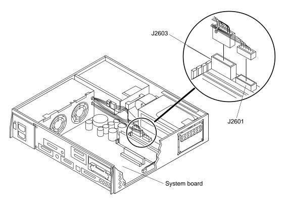
FIGURE 10-1 DC Power Disconnection
