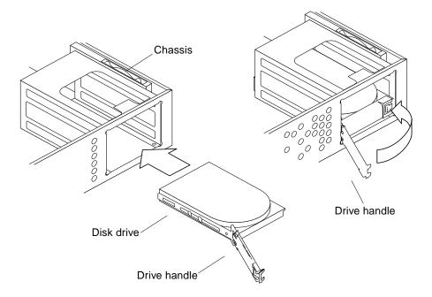
FIGURE 9-3 Replacing the Disk Drive
