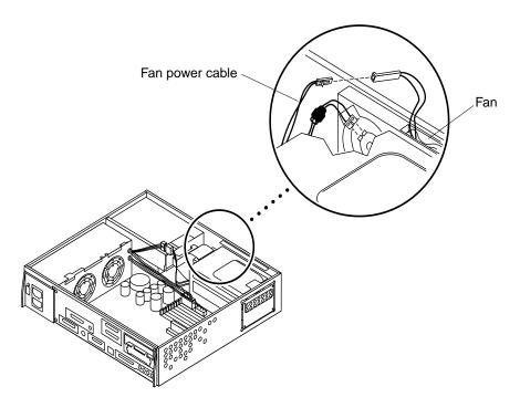
FIGURE 8-4 Fan Power Cable Connection
