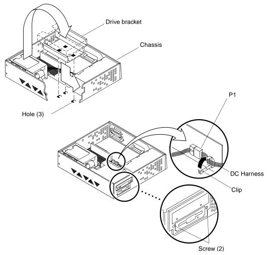
FIGURE 8-27 Replacing the Drive Bracket
