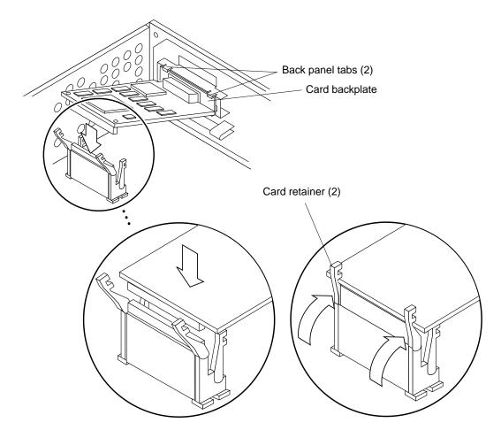
FIGURE 10-15 Replacing the SBus Card
