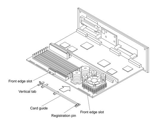
FIGURE 10-6 Installing the Card Guide
