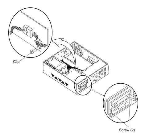
FIGURE 8-22 Removing the Drive Bracket
