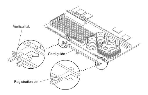
FIGURE 10-5 Card Guide Exploded view
