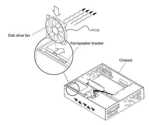
FIGURE 8-6 Replacing the Disk Drive Fan
