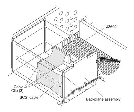
FIGURE 8-15 Removing the Backplane Assembly
