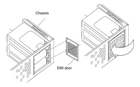
FIGURE 9-4 Replacing the EMI Door
