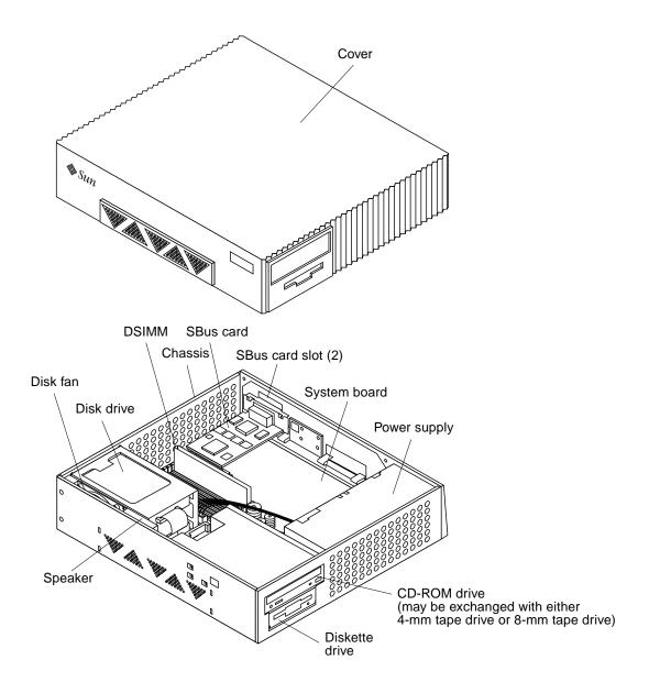
FIGURE 1-4 System Unit with Cover Removed
