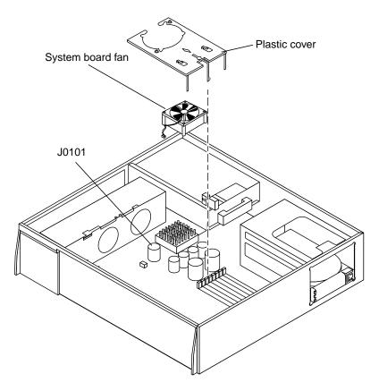
FIGURE 10-25 System Board Fan
