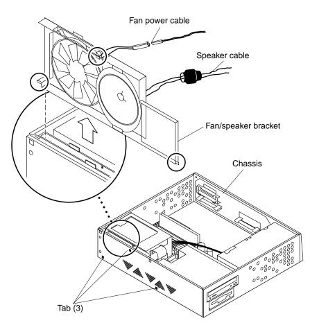
FIGURE 8-10 Replacing the Fan/Speaker Bracket
