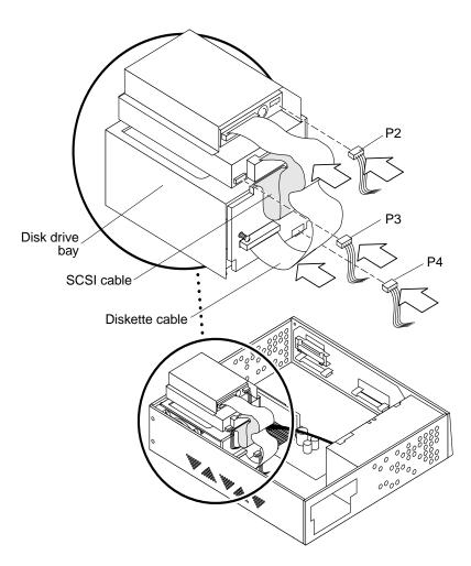
FIGURE 8-20 Replacing the Peripheral Power Cable Connection
