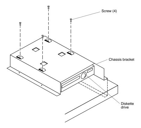
FIGURE 9-10 Positioning the Diskette Drive
