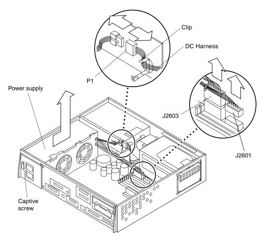
FIGURE 8-1 Removing the Power Supply
