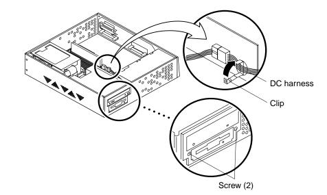
FIGURE 8-21 Replacing the Drive Bracket
