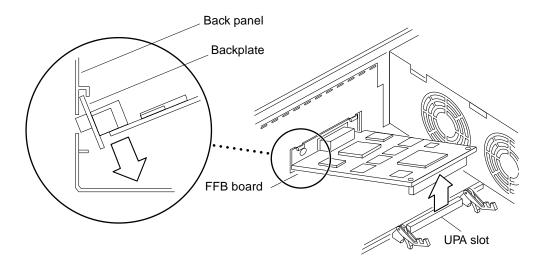
FIGURE 10-17 Removing the FFB Card
