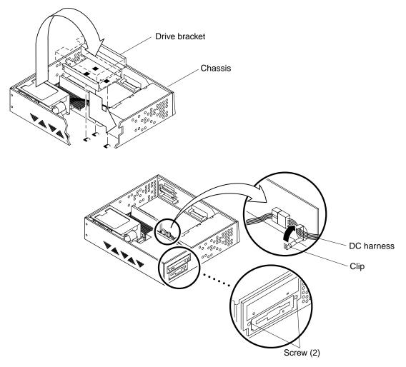
FIGURE 8-13 Replacing the Drive Bracket
