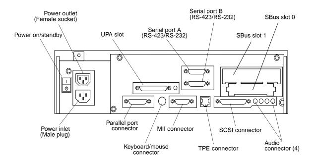
FIGURE 1-3 System Unit Rear View
