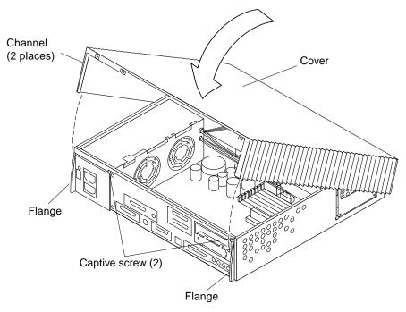
FIGURE 7-4 Replacing the Cover
