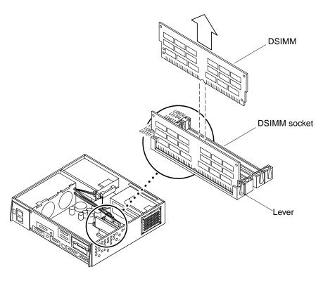
FIGURE 10-22 Removing a DSIMM
