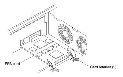
FIGURE 10-20 Securing the FFB Card Into the Chassis
