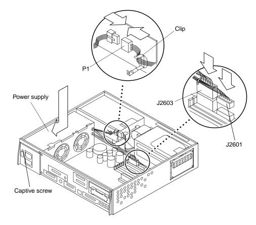
FIGURE 8-3 Securing and Connecting the Power Supply
