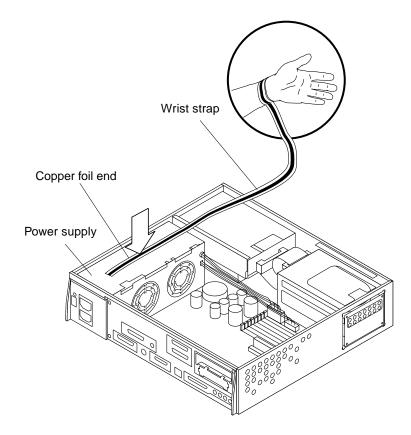
FIGURE 7-3 Attaching the Wrist Strap
