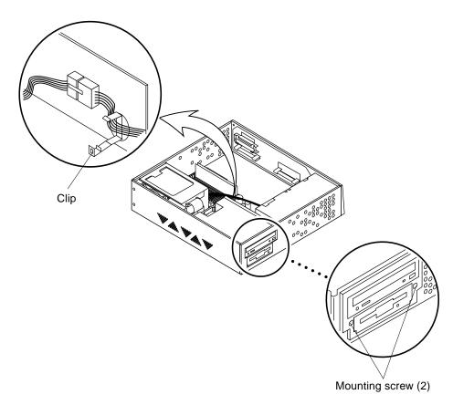
FIGURE 8-11 Removing the Drive Bracket
