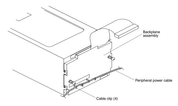
FIGURE 8-19 Backplane Assembly Peripheral Power Cable Routing
