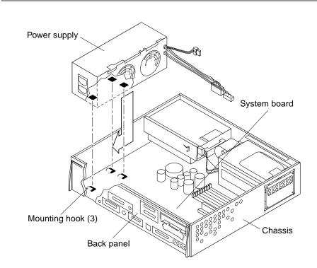
**Note** – Ensure that the hooks located on the chassis base engage with the cutouts located on the bottom of the power supply.
