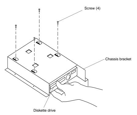
FIGURE 9-11 Positioning the Diskette Drive
