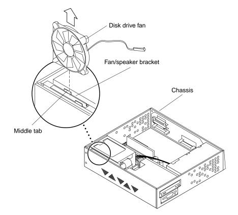
b. Grasp the fan and pull it from the fan/speaker bracket.
