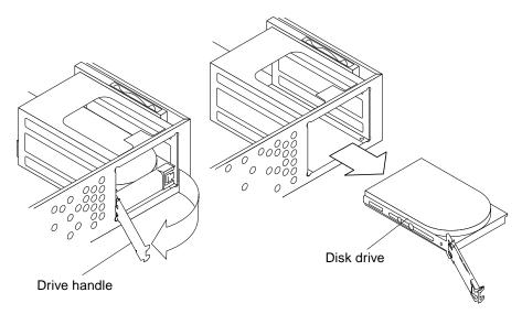
FIGURE 9-2 Removing the Disk Drive
