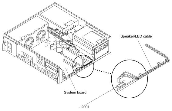
FIGURE 8-26 Speaker Connector on the System Board
