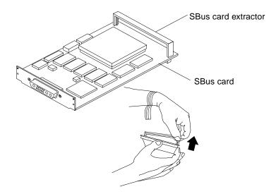
FIGURE 10-14 Removing the SBus Card Extractor
