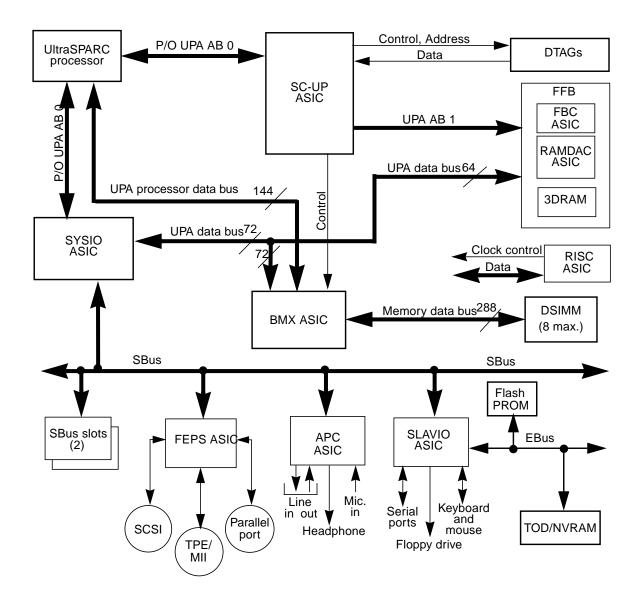
FIGURE C-1 System Unit or Server Functional Block Diagram
