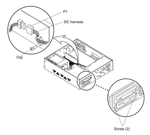
FIGURE 9-5 Chassis Bracket
