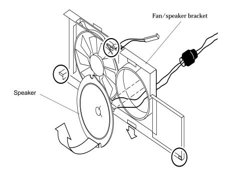
FIGURE 8-9 Removing the Speaker from the Fan/Speaker Bracket
