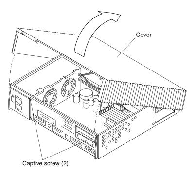
FIGURE 7-2 Removing the Cover
