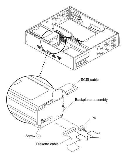
FIGURE 8-14 SCSI/Backplane Assembly Cable Connection
