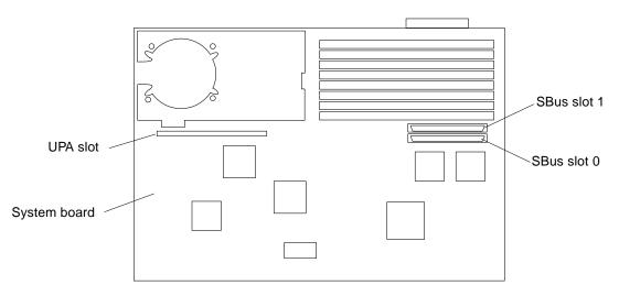
FIGURE 10-12 SBus Slot Locations.
