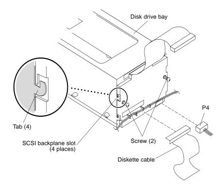
FIGURE 8-16 Replacing the SCSI Backplane
