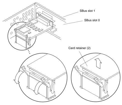
FIGURE 10-13 Removing an SBus Card from Slot 0 or 1
