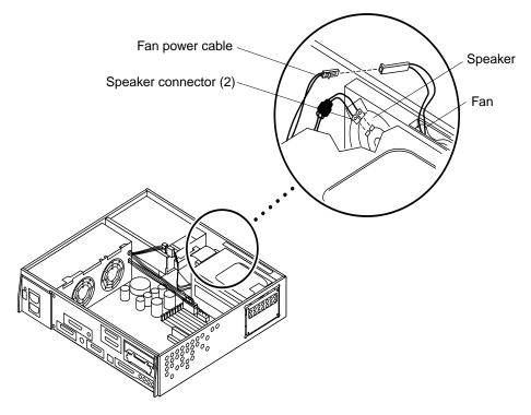
FIGURE 8-7 Fan and Speaker Cable Connection
