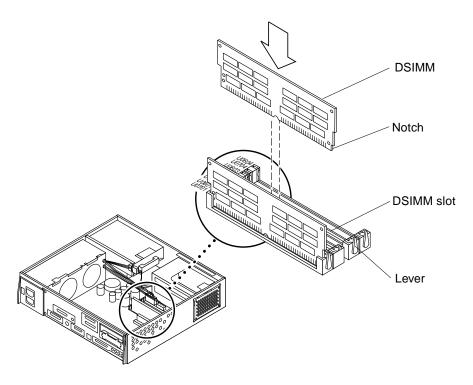
FIGURE 10-23 Installing a DSIMM
