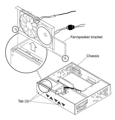
FIGURE 8-8 Removing the Fan/Speaker Bracket
