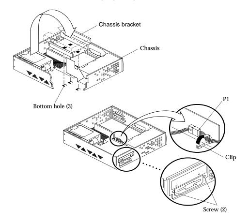
FIGURE 9-8 Positioning the Chassis Bracket
