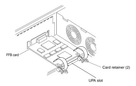
FIGURE 10-16 Preparing to Remove the FFB Card
