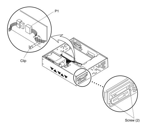
FIGURE 8-17 Removing the Drive Bracket
