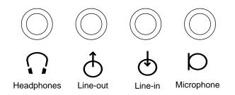
FIGURE B-5 Audio Connector Configuration
