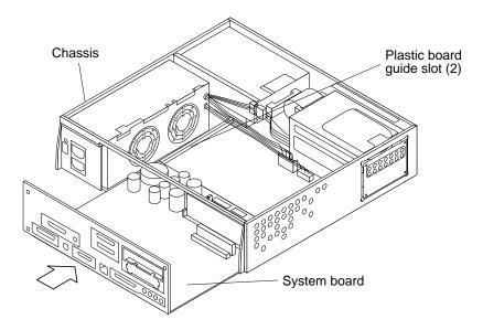
FIGURE 10-7 Sliding the System Board Into The Chassis
