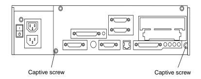
FIGURE 10-2 Captive Screws on the Back Panel
