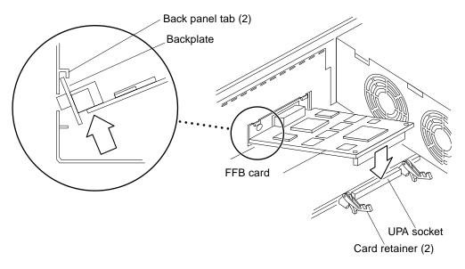
FIGURE 10-18 Replacing the FFB Card
