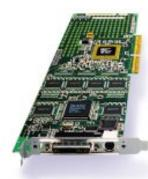
In medical imaging applications, Creator3D handles 3-D geometries and uses VIS for accelerated imaging, scaling, interpolation, and display of 2-D images and volumetric data.
