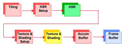
Figure 5. PowerVR Second Generation Rendering Pipeline
