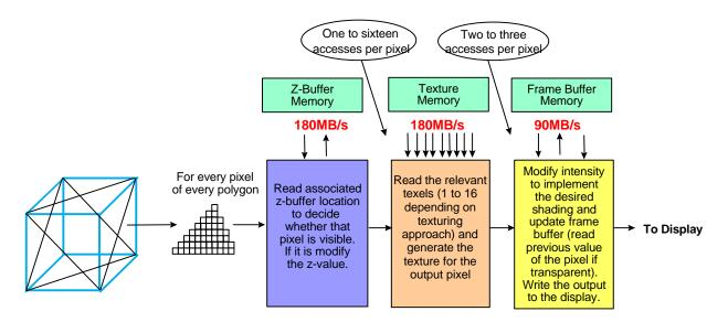
Figure 3. Data Flow in a Simplified Rendering Pipeline at 500K polygons/sec
