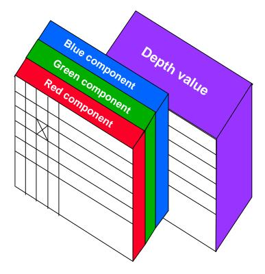
Figure 2. Representation of Z Buffer
