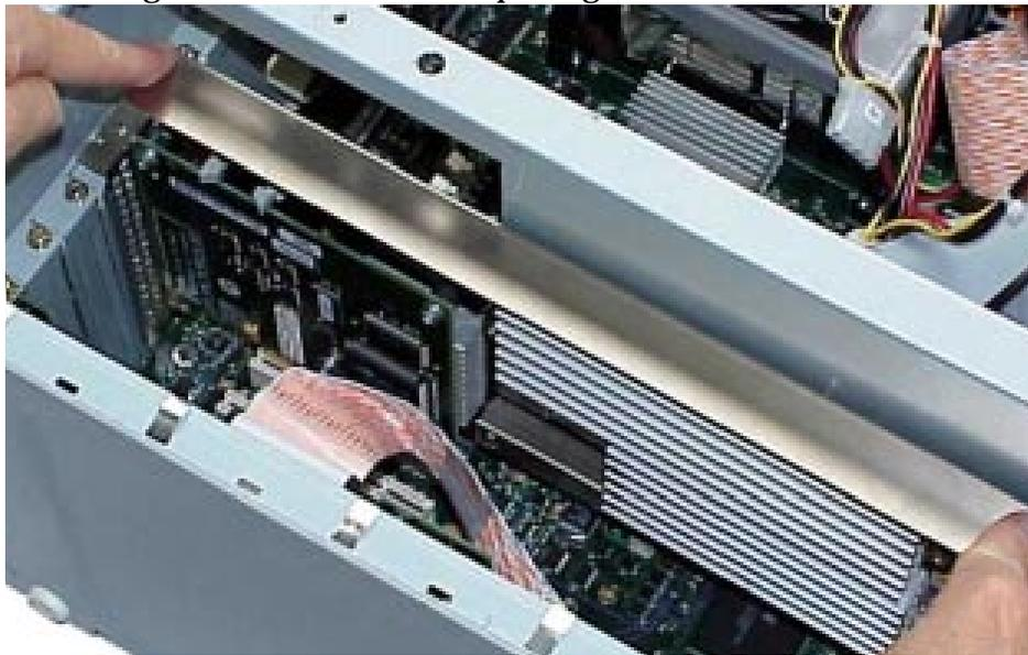
3. Align the cards's AGP contact fingers and PCI contact fingers with their appropriate system board connector slots and push the card firmly into position.
