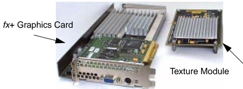
1. Remove the two screws from the card's strengthening bar, and then remove the strengthening bar from the HP VISUALIZE *fx+* Graphics Card. (You can use a Torx™ screwdriver or a flat-blade screwdriver of the correct size.)
