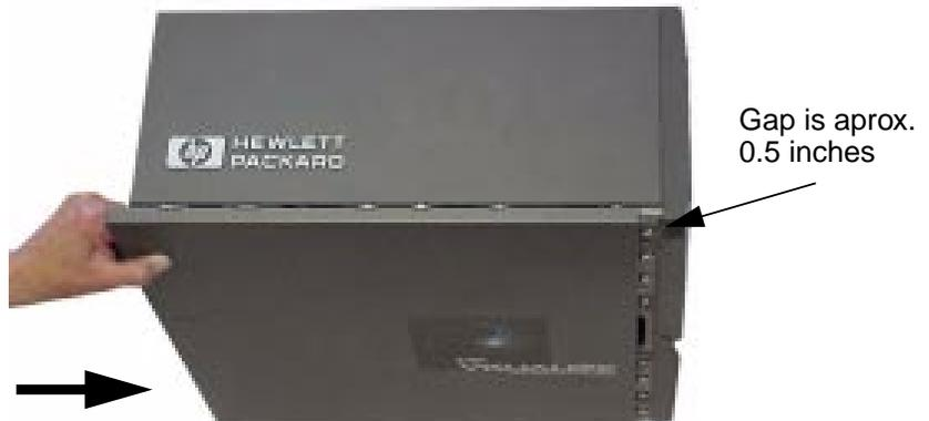
3. Screw the left-side panel thumb screws in place to complete the left-side panel replacement on the Personal Workstation.
