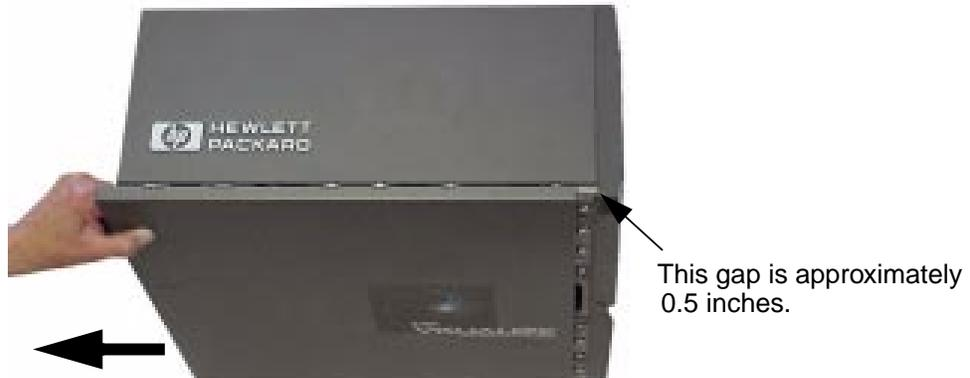
3. Remove the left-side panel by grasping the rear part of the panel as shown in Figure 1-3 and pulling the panel outward. Next, lift the panel up and away from the Personal Workstation, and place it where its exterior surface cannot be damaged.
