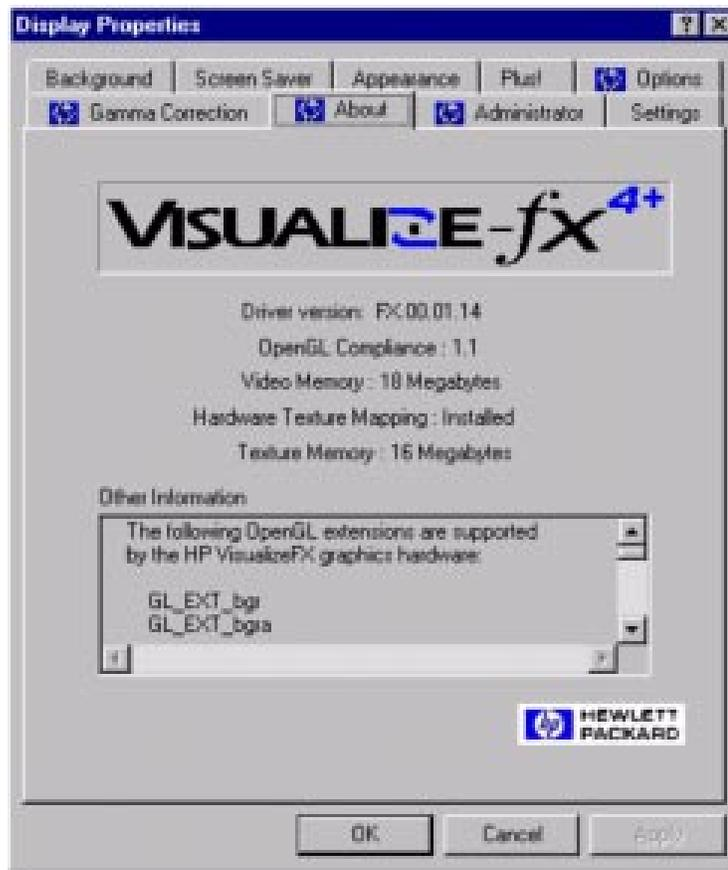
The figure above shows the **About** panel for an HP VISUALIZE *fx+* Graphics card with driver version FX.00.01.14 and a 16 MByte texture memory module installed.
