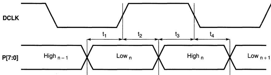
**Figure 7-36. P-Bus as Inputs: 16-Bit Mode (External DCLK)**
