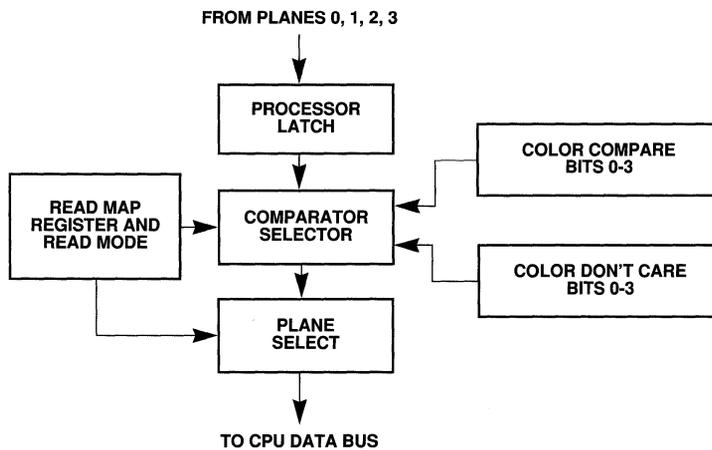
Figure 2-3. Graphics Controller Read Operation
