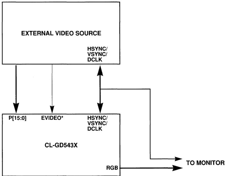
Figure B14-2. Switch with EVIDEO\*
