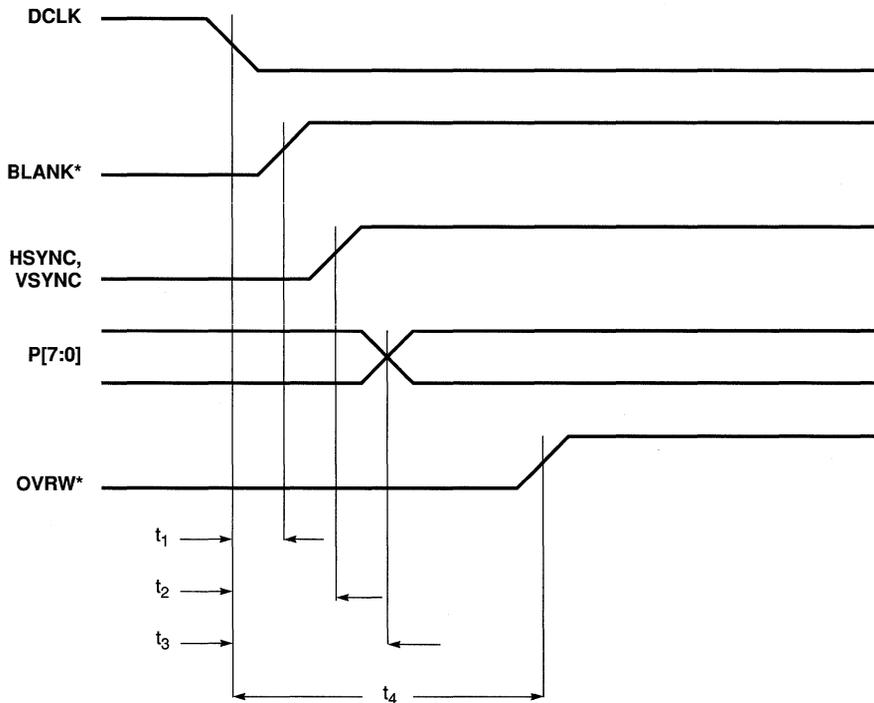
**Figure 7-32. Feature Bus Timing: 8-Bit Mode, Outputs (Internal DCLK)**
