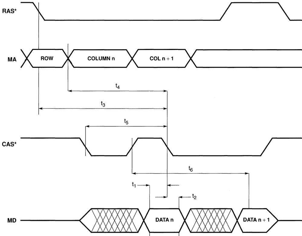
**Figure 7-29. Display Memory Bus: Read Cycles (EDO Timing — CL-GD5436)**
