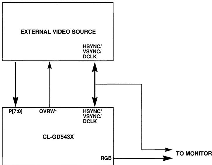
**Figure B14-4. Switch with OVRW\***
