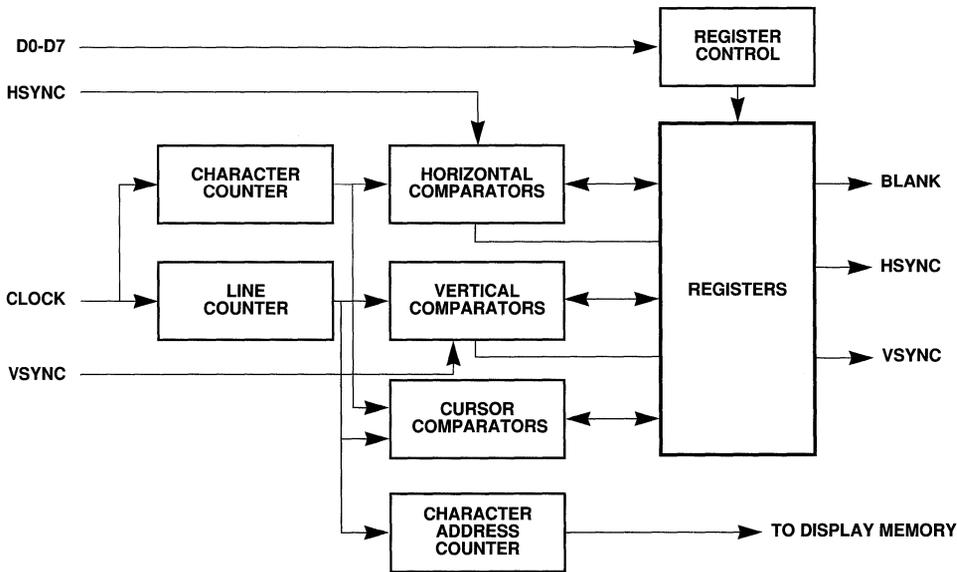
Figure 2-1. CRT Controller Functional Block Diagram
