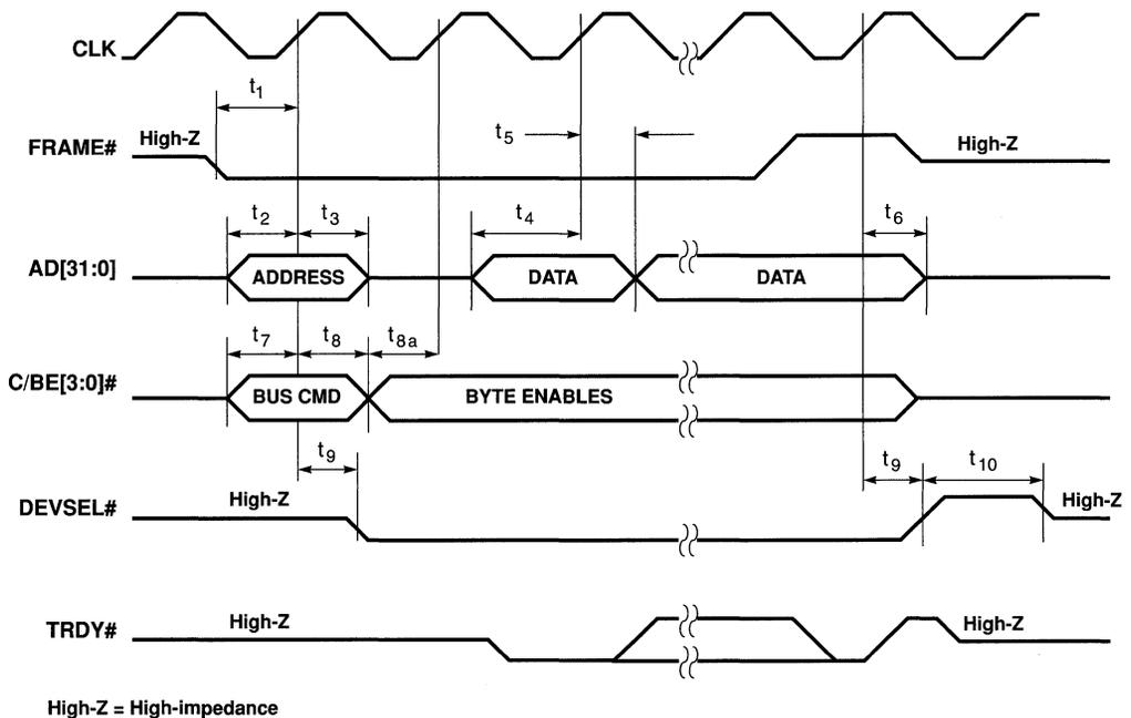
Figure 7-17. FRAME#, DEVSEL#, AD[31:0], and C/BE[3:0]# (PCI Bus)
