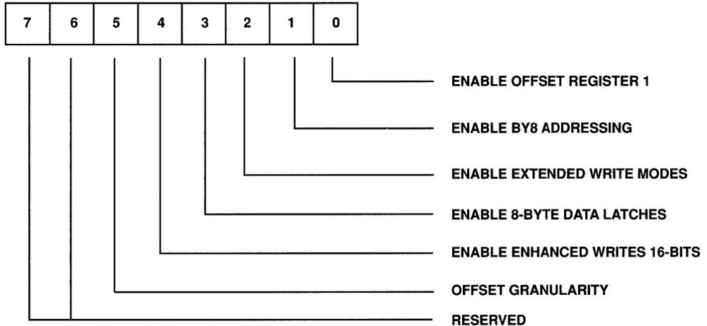
**Figure D1-7. Extension Register GRB**
