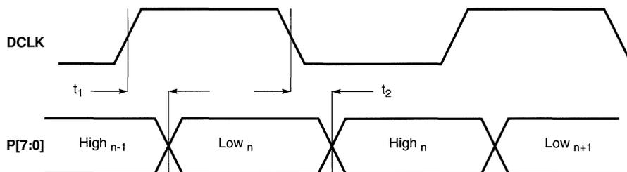
**Figure 7-33. P-Bus as Outputs: 16-Bit Mode (Internal DCLK)**
