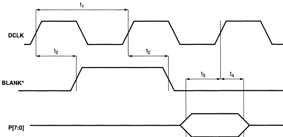
**Figure 7-38. Video Port Timing: Detail (CL-GD5440 only)**
