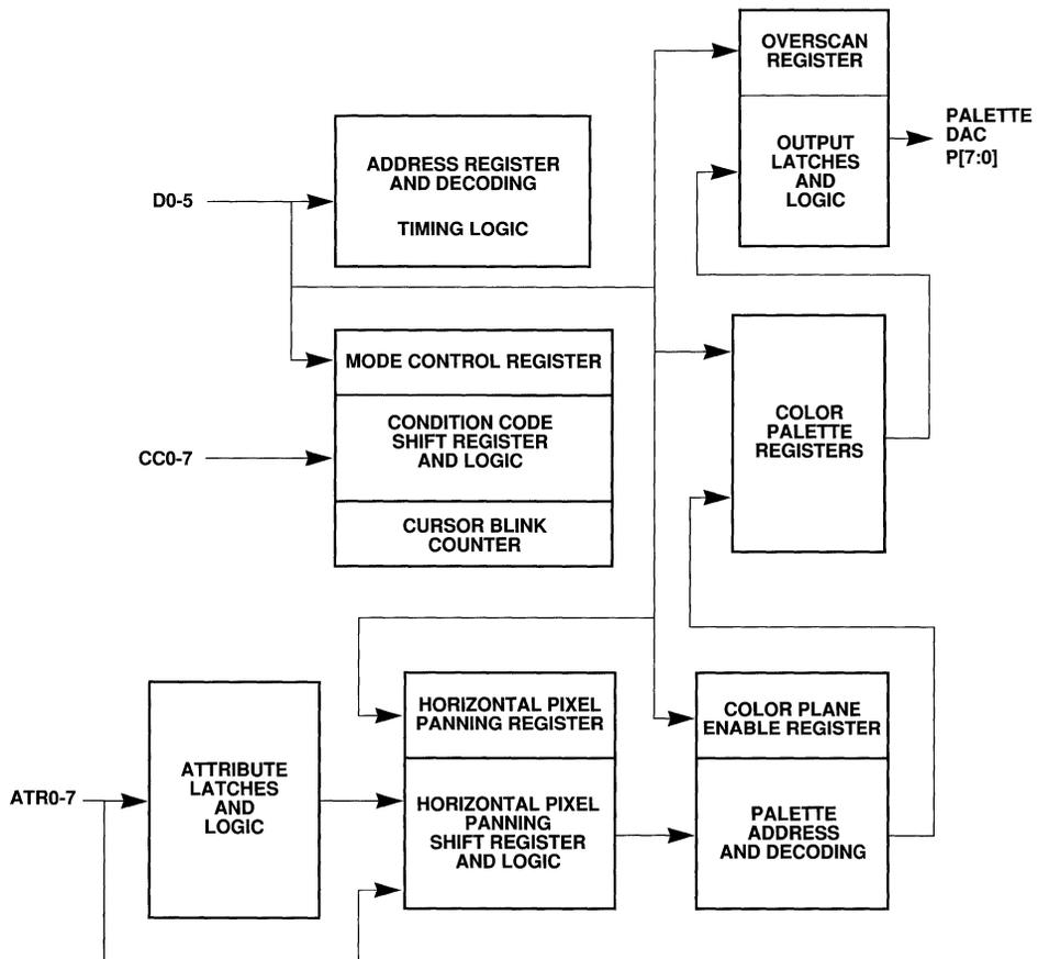
**Figure 2-4. Attribute Controller Functional Block Diagram**
