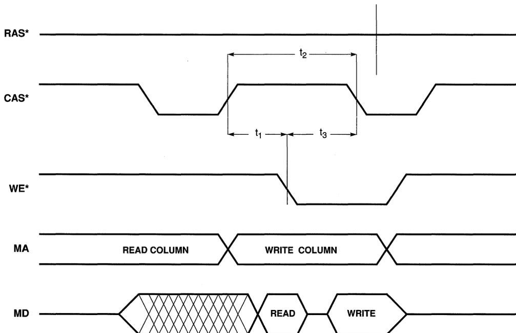
**Figure 7-30. Display Memory Bus: BitBLT R-W Cycle (CL-GD5436 only)**
