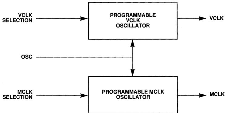
**Figure 2-5. Programmable Dual-Frequency Synthesizer Functional Diagram**
