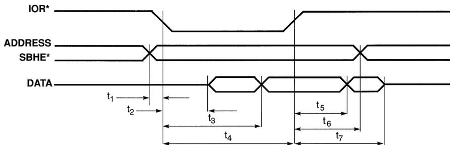
Figure 7-2. I/O Read Timing (ISA Bus — CL-GD5434 only)
