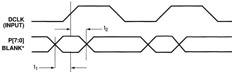
**Figure 7-31. P-Bus as Inputs: 8-Bit Mode (External DCLK)**
