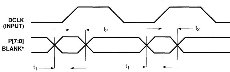
**Figure 7-35. P-Bus as Inputs: 16-Bit Mode, Clock Mode 2 (External DCLK)**
