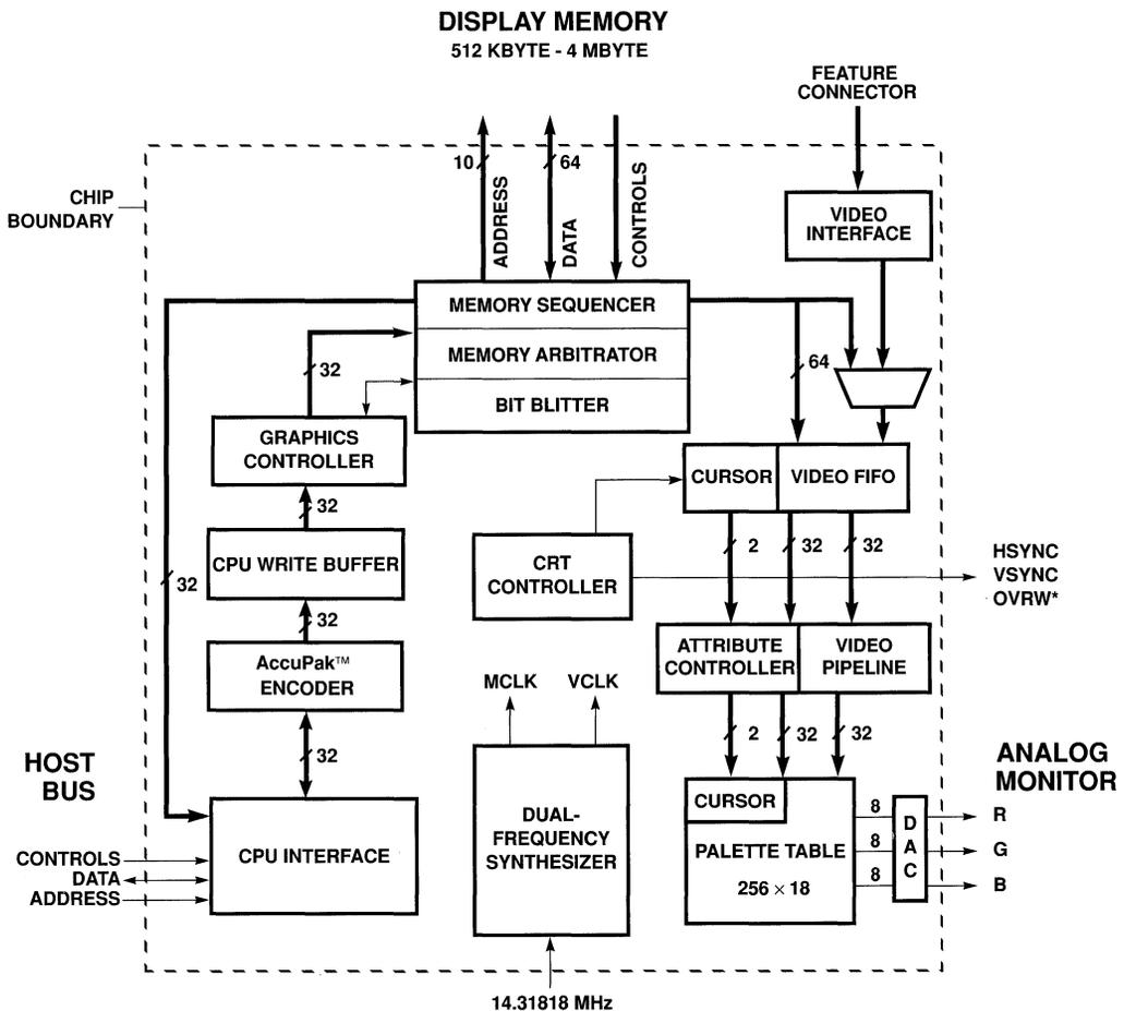
Figure 3-1. CL-GD543X/4X Chip Block Diagram
