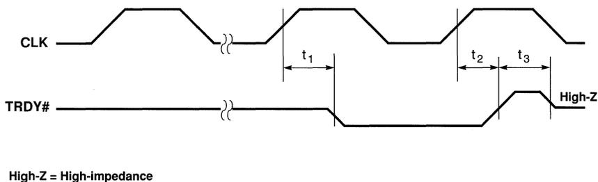
**Figure 7-18. TRDY# Delay (PCI Bus)**
