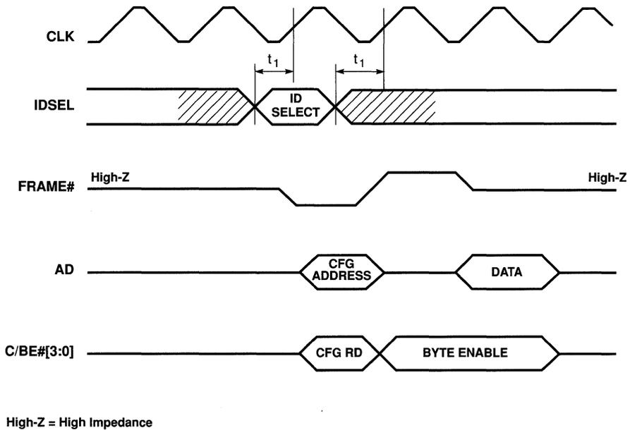
Figure 7-21. IDSEL Timing (PCI Bus)
