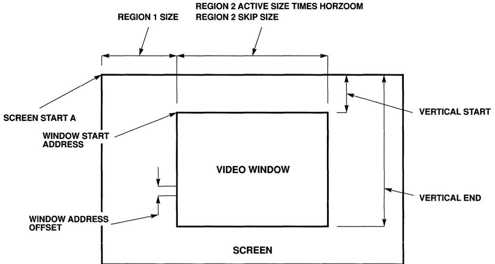
The following table specifies the registers that control the video window and indicates how they relate to the above diagram.
