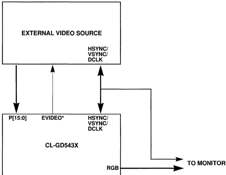
Figure B14-3. Switch with Color Key
