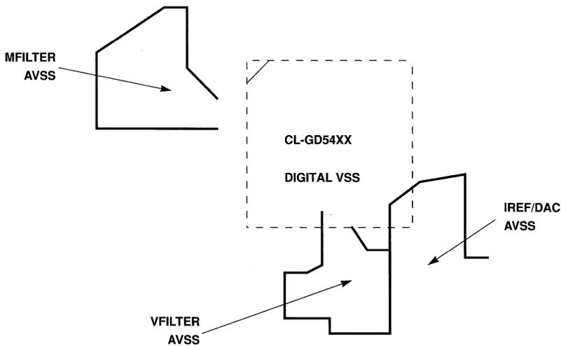
**Figure B12-5. Ground Plane Layout**
