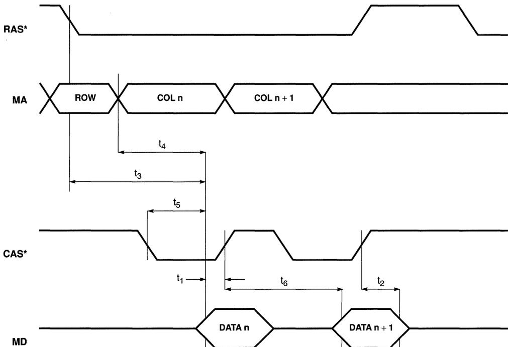
**Figure 7-26. Display Memory Bus: Read Cycles**
