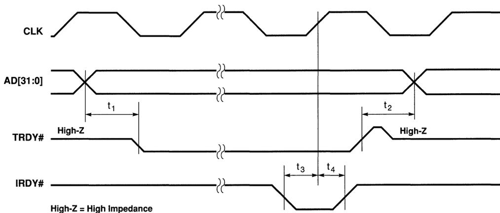
Figure 7-19. Read Data/IRDY# (PCI Bus)
