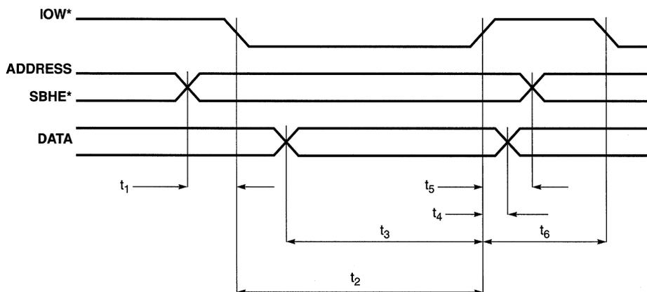
**Figure 7-1. I/O Write Timing (ISA Bus — CL-GD5434 only)**
