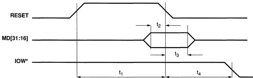
**Figure 7-40. RESET Timing**
