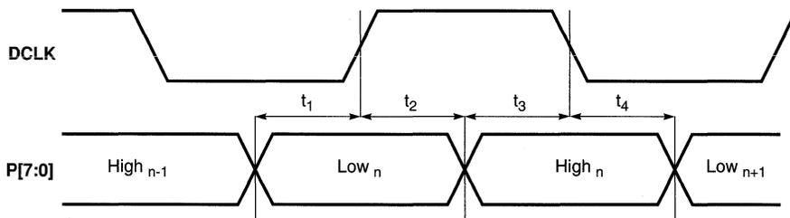
**Figure 7-34. P-Bus as Inputs: 16-Bit Mode (External DCLK)**
