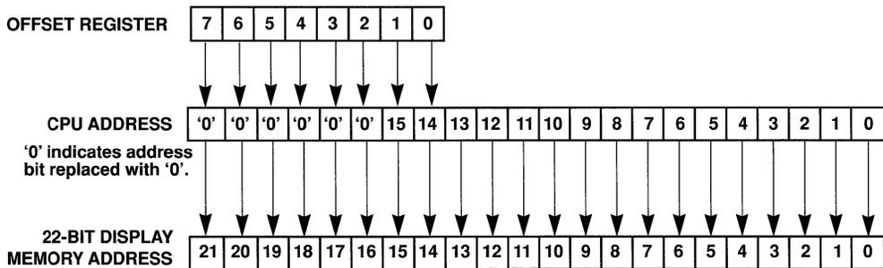
Figure D1-4. Single Page Mode Remapping Adder Alignment with 16-Kbyte Granularity
