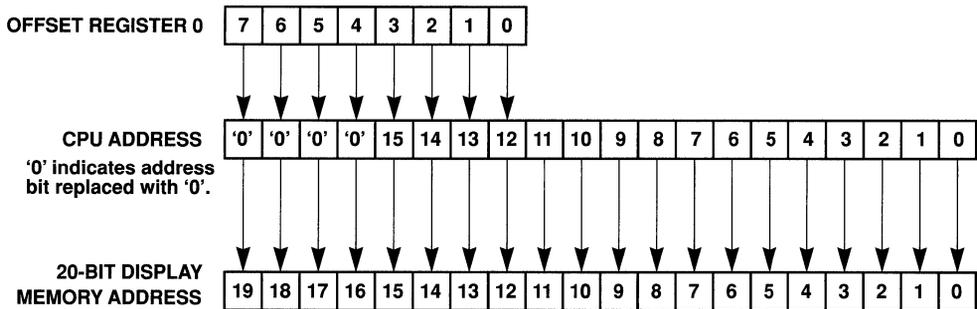
Figure D1-3. Single Page Mode Remapping Adder Alignment with 4-Kbyte Granularity
