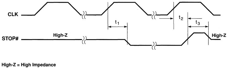
**Figure 7-20. STOP# Delay (PCI Bus)**
