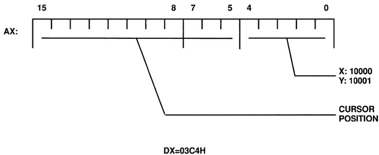
Figure D1-1. Cursor Position Programming
