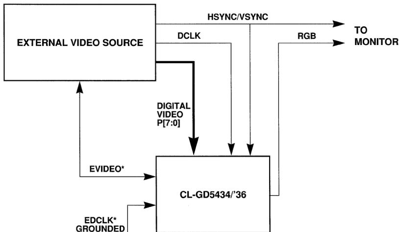
Figure B17-1. Video Overlay Connections
