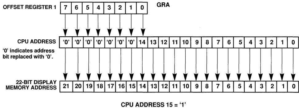
Figure D1-6. Dual-Page Mode Remapping Adder Alignment with 16-Kbyte Granularity
