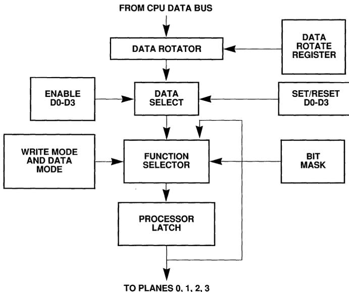
Figure 2-2. Graphics Controller Write Operation
