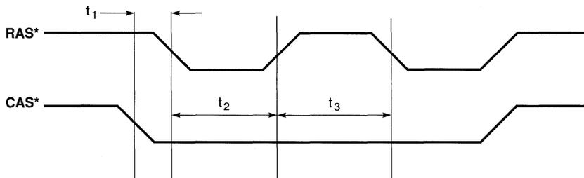
**Figure 7-24. CAS\*-before-RAS\* Refresh Timing (Display Memory Bus)**
