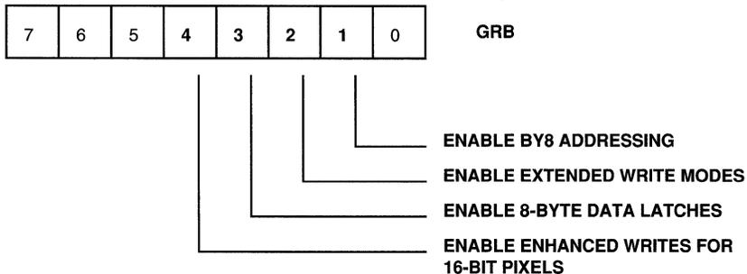
Figure D6-1. Color Expansion Controls
