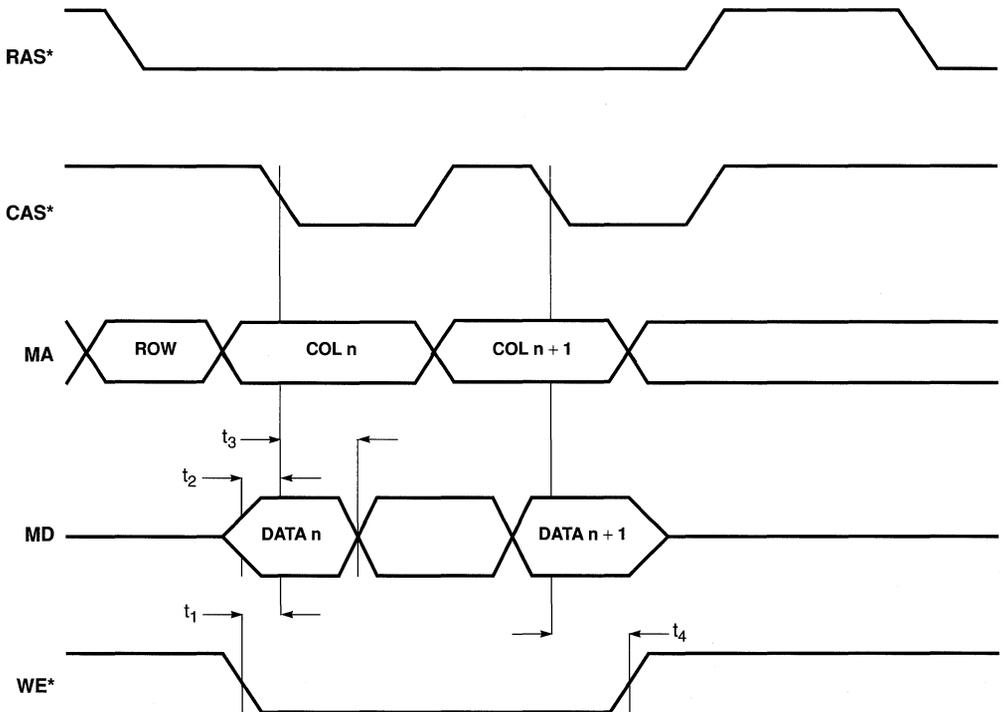
**Figure 7-27. Display Memory Bus: Write Cycles**
